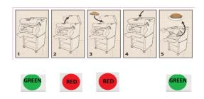
A)When the machine is ready to work the indicator light is green so you can open the upper cover and put the bread inside
